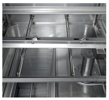
The DOUBLE "DR" RINSE system is standard in the TS series: the final rinse water is not wasted, but is recovered in the rinse tank and used to supply a pre-rinse zone at controlled pressure by the internal pressure booster pump. Rinsing is done at constant and optimum pressures and temperatures whatever the pressure of the mains water supply.
