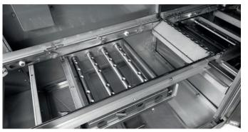
Pre-wash, washing and rinse arms made of stainless steel that are easy to dismantle and inspect without having to use any tools.
